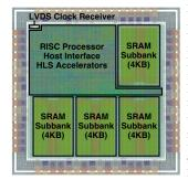
Figure 1. **BRGTC1 Test Chip** – A taped-out  $2 \times 2 \text{ mm } 1.3 \text{ M-transistor}$ test chip in IBM 130 nm designed and implemented using our new PyMTL hardware modeling framework. Chip includes a simple pipelined 32-bit RISC processor, custom LVDS clock receiver, 16 KB of on-chip SRAM, and application-specific accelerators generated using commercial C-to-RTL high-level synthesis tools.
