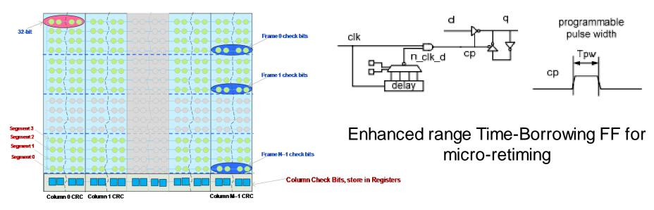
Column based CRAM CRC on top of Row Based Up to 100x Faster Error Detection and Correction
