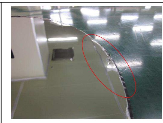
→ Adhesive squeeze out
