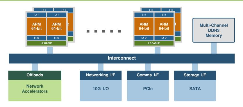
64bit ARM Server Class CPU → Multi-core for Distributed Computing
