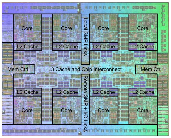
POWER7<sup>™</sup> is an 8-core, high performance Server chip. A solid chip is a good start. But to win the race, you need a balanced system. POWER7 enables that balance.
