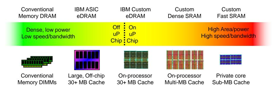
Industry Standard Caching and Memory Technologies: Conventional DIMMs, Dense and Fast SRAM's.
