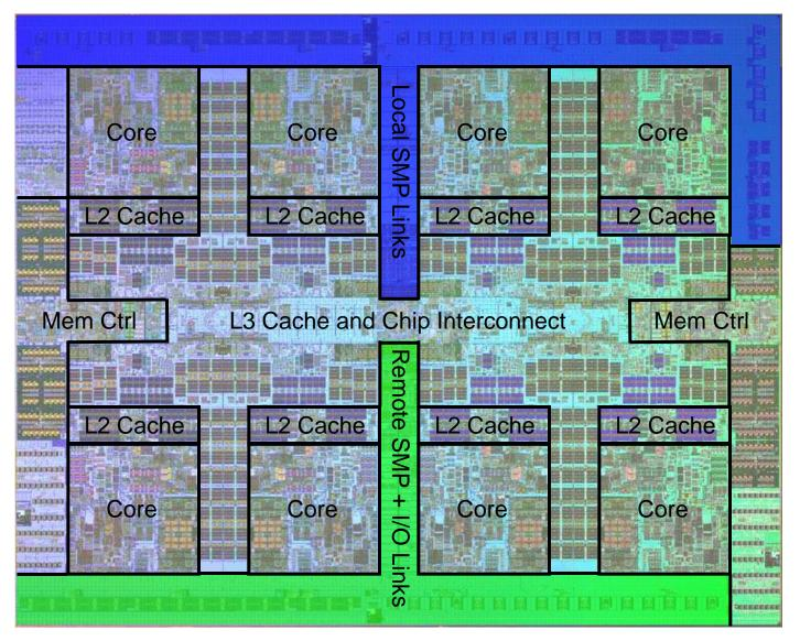
Using local and remote SMP links, up to 32 POWER7 chips are connected
