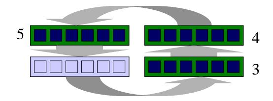
Since stripes are connected in a ring, data can always pass between adjacent virtual stripes in the physical fabric.
