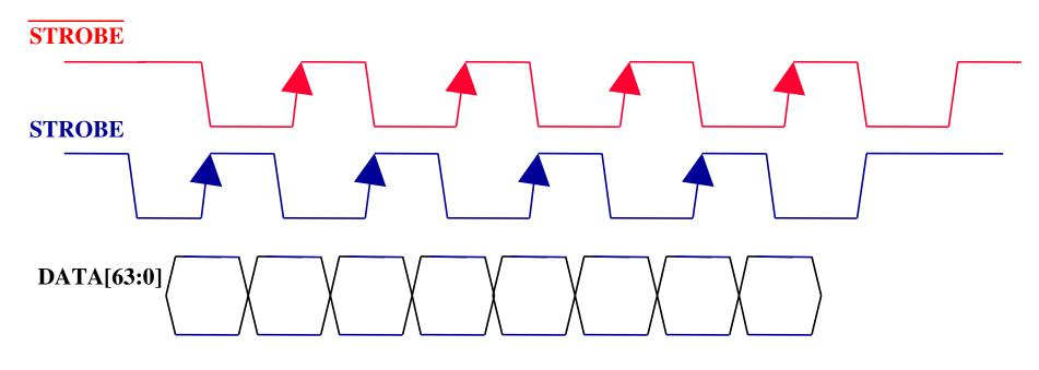
**Note: STROBE and <b>STROBE** are the Source Synchronous clocks
