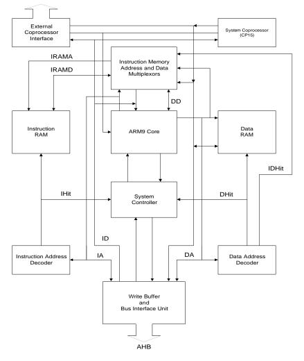
• Tightly coupled instruction and data RAM - variable size up to 64M. RAM fixed in memory map to ease implementation and reduce power.
