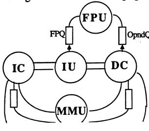
The FPU runs in parallel with the IU. A queue caries Floating Point Instructions to the FPU; an Operand Queue carries data values from the data cache to the FPU.
