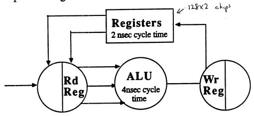
In the second half of a clock, we read two values from the register banks. In the next clock, these values are operated on by the ALU. In the first half of the next clock, the result is written to the register bank
