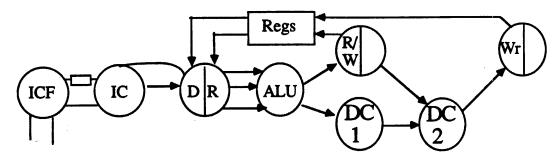
The data cache lives in the pipe after the ALU. One cycle is needed for lookup, and another for a store. On a load, DC provides its value to a second Register Write stage. On a store, the normal RegWrite stage sources a value.
