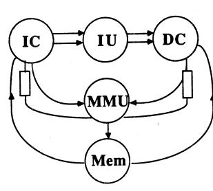
The MMU accepts requests from the Icache and Dcache. Dcache has absolute priority. MMU produces a 36 bit physical address from the 32 bit virtual address. A queue of requests is built by the MMU back to each cache. MMU is cache-like, walks own 2-level page tables. An 8-bit context number is hashed with the virtual address.
