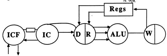
The icache provides two instructions at a time to the Decode stage. On a miss, it can queue up many requests to the memory system
