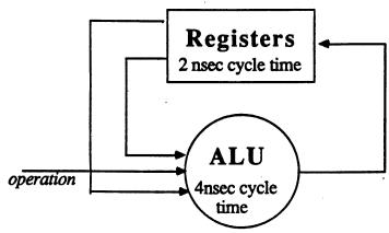
to get one instruction per clock, we must pipeline register read, alu operation and register write
