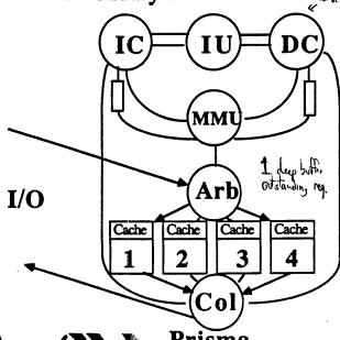
The secondary cache is a 4-way interleaved design; each bank can be active simultaneously. An Arbitrator between the MMU and the cache banks also shares cache bandwidth between CPU and IO traffic. A collector behind the cache banks provides data in the correct order to the requestors.
