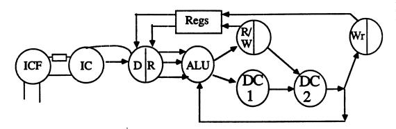
To reduce the latency caused by the 2-stage cache pipe, results are forwarded to the ALU in parallel with being written to the registers. This provides performance similar to a single cycle cache at the cost of design complexity
