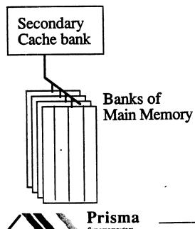
Because the main memory banks are only ever accessed by the secondary cache, advantage may be taken of the relatively long transfers needed to read and write its cache lines. This allows the use of DRAM with little performance penalty
