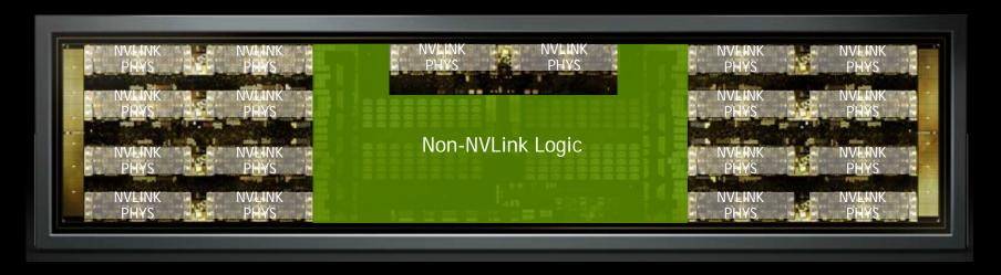
Packet-processing and switching (XBAR) logic is extremely compact
